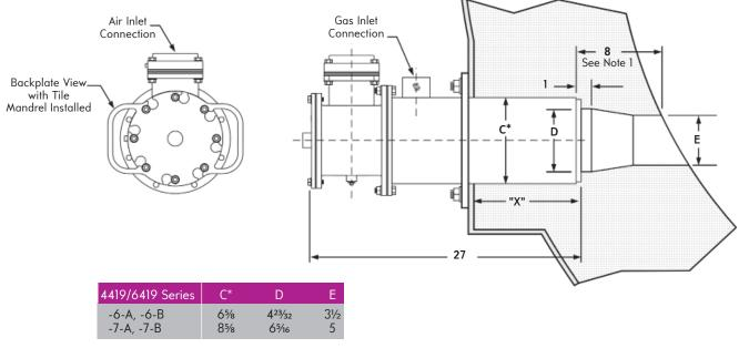
\* C = diameter of outer burner tube (becomes part of mandrel during installation).
