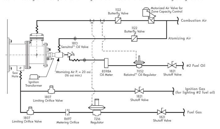
**NOTE:** Gas connection is shown at bottom for clarity. Whenever possible gas and air connections should not be located at the bottom of the burner on dual fuel applications.
